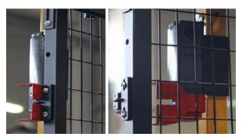
(\*) the fixing systems (screws) are in accordance with table 3 of the UNI EN 14119
