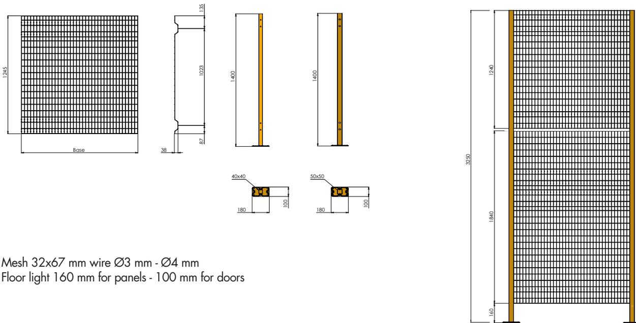
Mesh 32x67 mm wire Ø3 mm - Ø4 mm
