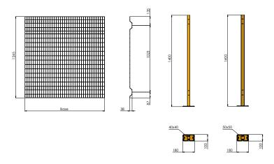
Mesh 32x67 mm wire  $\emptyset 3$  mm -  $\emptyset 4$  mm Floor light 160 mm for panels - 100 mm for doors
